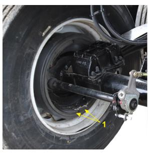
Figure 4-12 – Brake Lining Inspection
