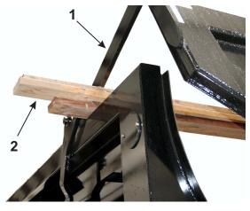
Figure 2-2 – Tailgate Lowered onto Wooden Blocking
