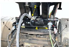
Figure 3-10 – Umbilical Connections from Tractor to Semitrailer
