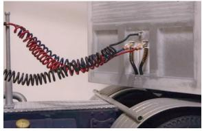
Figure 4-11 – Properly Supported Air and Brake Lines
