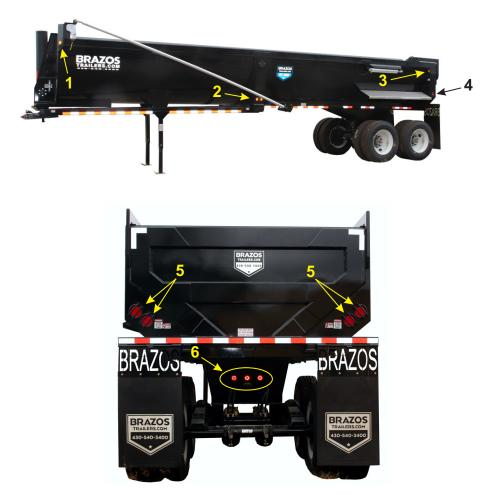
Figure 3-19 – Semitrailer Marker, Stop and Turn Signal Lights
