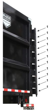
Figure 4-10– Manual Tailgate Grease Zerks
