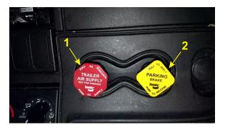
Figure 3-12– Tractor Air Supply Controls
